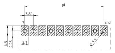
Stencil thickness: 120 µm
