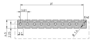
Stencil thickness: 120 µm
