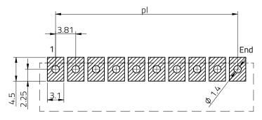
Stencil thickness : 120 µm
