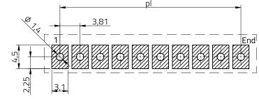
Stencil thickness : 120 µm
