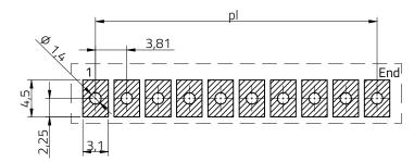
Stencil thickness: 120 µm
