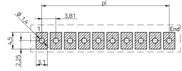
Stencil thickness : 120 µm
