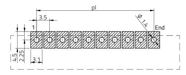
Stencil thickness: 120 µm
