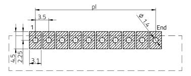
Stencil thickness: 120 µm
