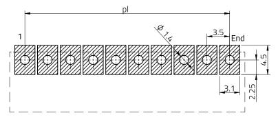
Stencil thickness: 120 µm
