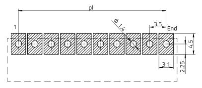
Stencil thickness: 120 µm
