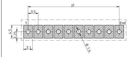
Stencil thickness: 120 µm
