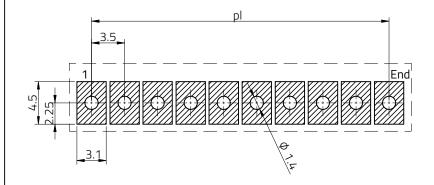
Stencil thickness: 120 µm
