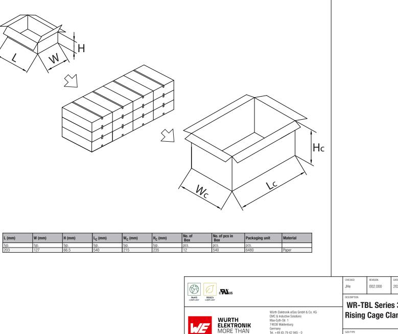
DATE (YYYY-MM-DD) GENERAL TOLERANCE PROJECTION METHOD Ð 2024-01-31 DIN ISO 2768-1m WR-TBL Series 3163 - Plug with **Rising Cage Clamp - Cable** ORDER CODE 691316310003 MORE THAN YOU EXPECT Tel. +49 (0) 79 42 945 - 0 www.we-online.com STATUS BUSINESS UNIT PAGE 3/5 3.81mm pitch - Modular Horizontal cable entry eiCan Valid eiSos@we-online.com
