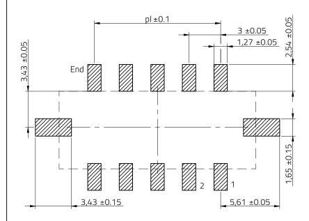
Recommended PCB thickness: 1.6 mm max.
