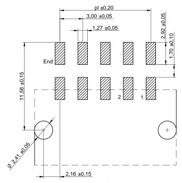
Max. Recommended PCB Thickness: 1.6mm
