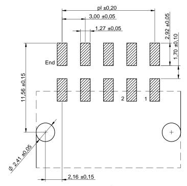
Max. Recommended PCB Thickness: 1.6mm
