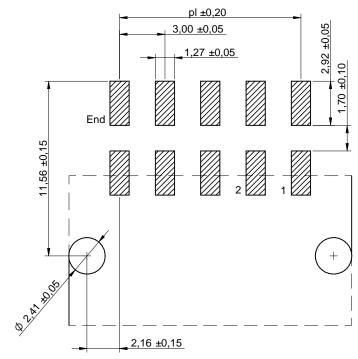
Max. Recommended PCB Thickness : 1.6mm
