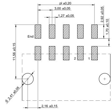
Max. Recommended PCB Thickness : 1.6mm
