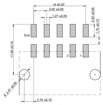
Max. Recommended PCB Thickness: 1.6mm
