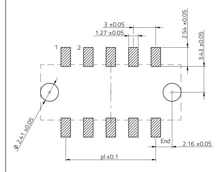
Max. Recommended PCB thickness: 1.6mm
