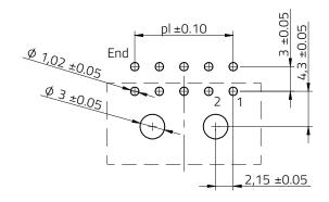
Max. Recommended PCB Thickness: 1.6mm
