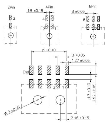
Max Recommended PCB Thickness: 1.6mm
