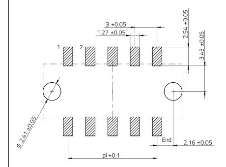
Max. Recommended PCB thickness : 1.6mm
