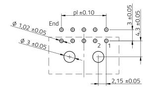
Max. Recommended PCB Thickness: 1.6mm
