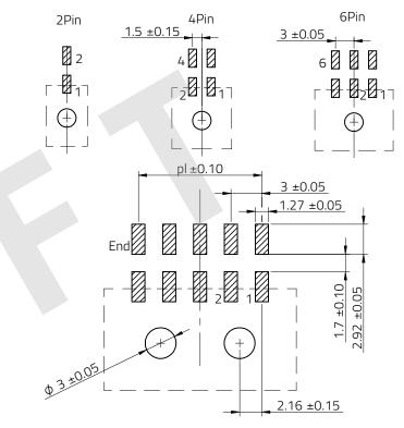
Max Recommended PCB Thickness : 1.6mm Scale - 2:1
