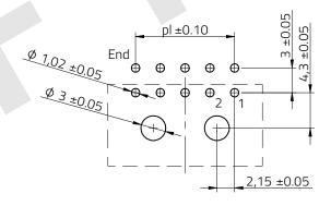
Max. Recommended PCB Thickness: 1.6mm
