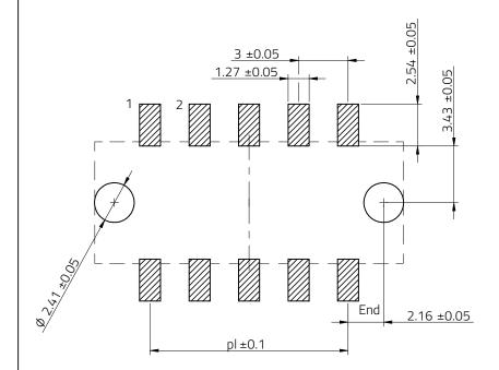
Max. Recommended PCB thickness : 1.6mm
