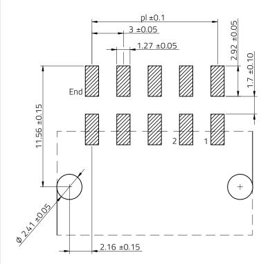
Max. Recommended PCB Thickness: 1.6mm
