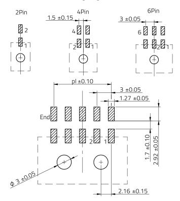
Max Recommended PCB Thickness: 1.6mm
