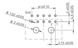
Max. Recommended PCB Thickness: 1.6mm
