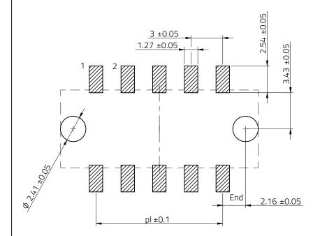
Max. Recommended PCB thickness : 1.6mm
