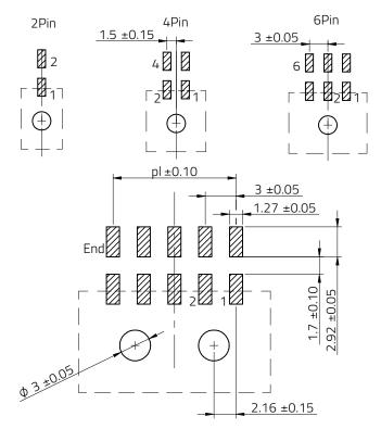
Max Recommended PCB Thickness: 1.6mm
