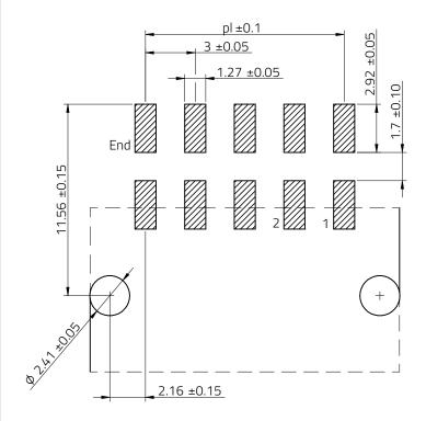
Max. Recommended PCB Thickness: 1.6mm
