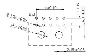
Max. Recommended PCB Thickness : 1.6mm
