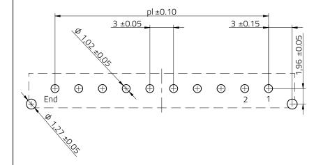
Max. Recommended PCB Thickness: 1.6mm
