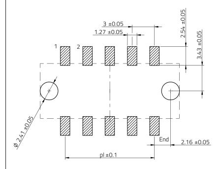
Max. Recommended PCB thickness: 1.6mm
