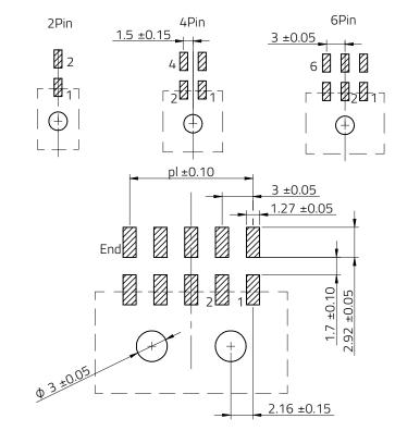
Max Recommended PCB Thickness : 1.6mm Scale - 2:1
