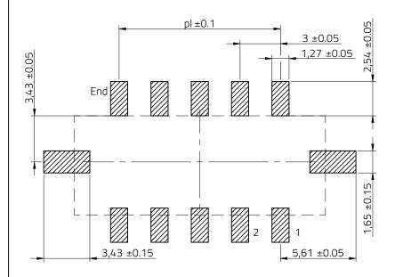
Recommended PCB thickness: 1.6 mm max.
