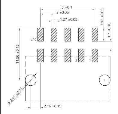
Max. Recommended PCB Thickness: 1.6mm
