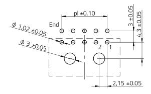
Max. Recommended PCB Thickness: 1.6mm
