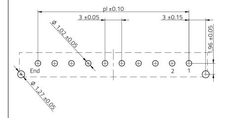
Max. Recommended PCB Thickness: 1.6mm
