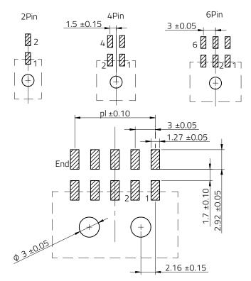
Max Recommended PCB Thickness: 1.6mm
