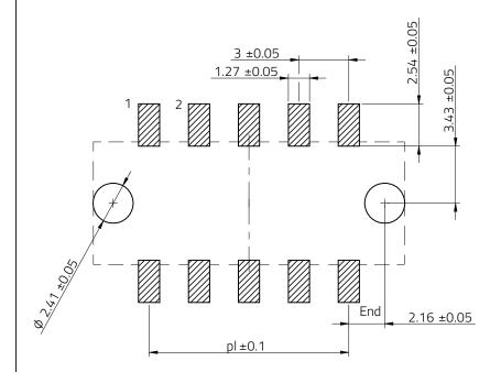
Max. Recommended PCB thickness : 1.6mm
