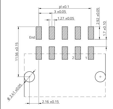
Max. Recommended PCB Thickness: 1.6mm
