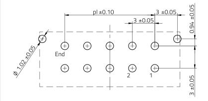
Max. Recommended PCB Thickness : 1.6mm
