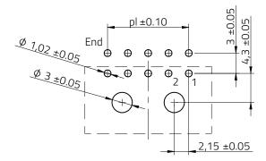
Max. Recommended PCB Thickness : 1.6mm
