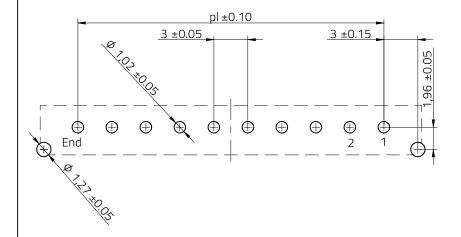
Max. Recommended PCB Thickness: 1.6mm
