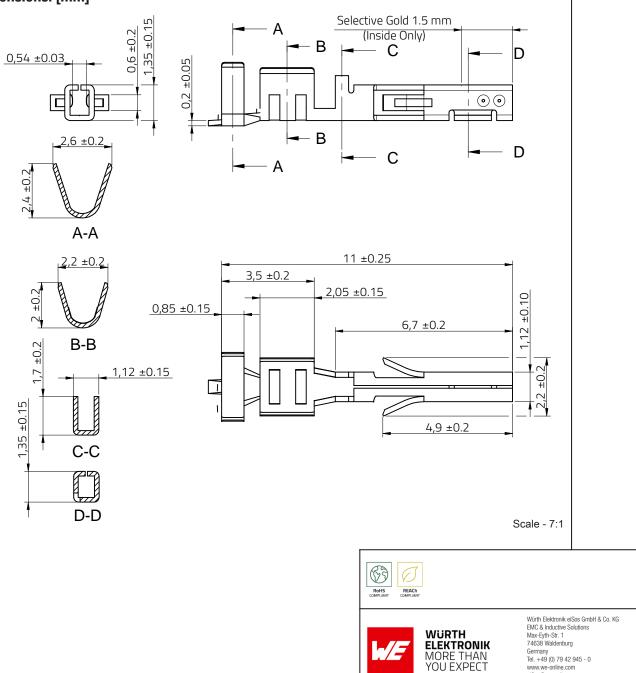
CHECKED REVISION DATE (YYYY-MM-DD) GENERAL TOLERANCE PROJECTION METHOD  $\oplus$ MPer 001.000 2023-06-23 DIN ISO 2768-1m DESCRIPTION **WR-MPC3 Female Crimp Terminal** ORDER CODE 66200113724DEC SIZE/TYPE BUSINESS UNIT STATUS PAGE AWG 24-20, Selective Gold Plating eiCan Valid 1/6
