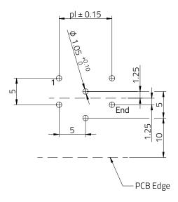
Recommended PCB Thickness: 1.6mm
