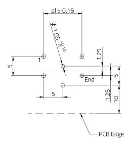
Recommended PCB Thickness: 1.6mm
